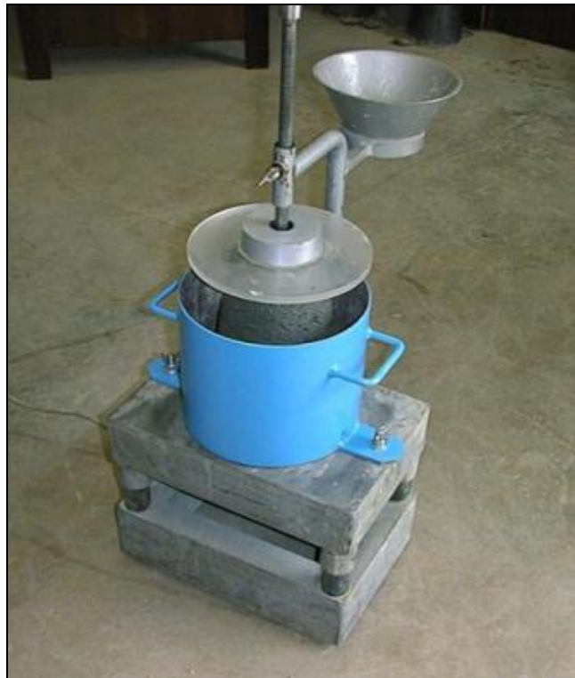
Figure 55. Vebe Test Equipment
